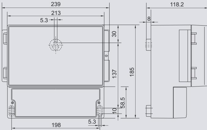
Please observe to have sufficient space (min. 30 mm) on the left-hand side of the transmitter to open the transparent door.
